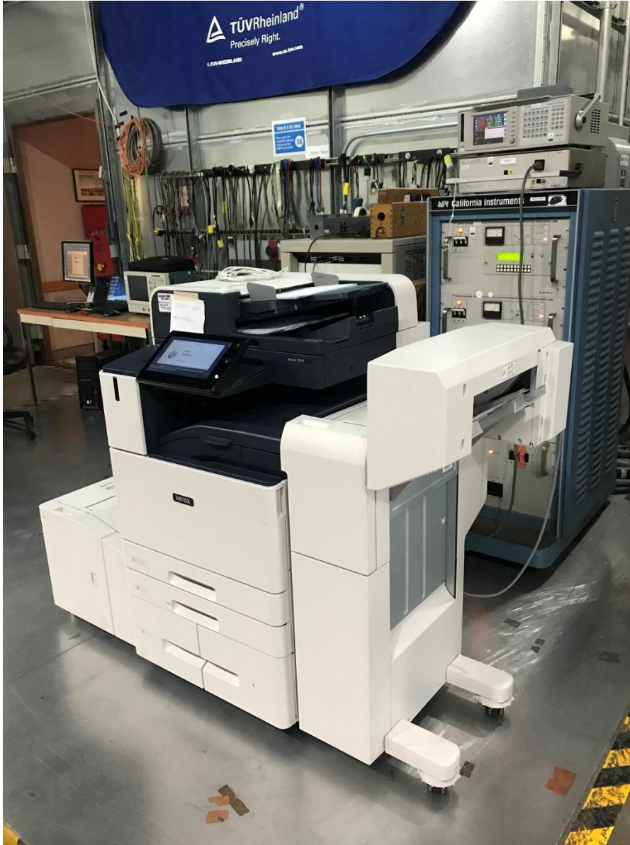
Figure 6 –Harmonic Current and Voltage Fluctuations & Flicker Test Setup
