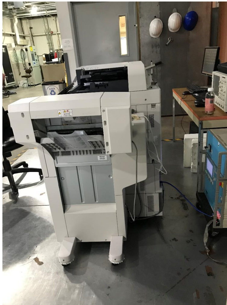
Figure 29 – Electrical Fast Transients (EFT) Immunity Test Setup AC Mains
